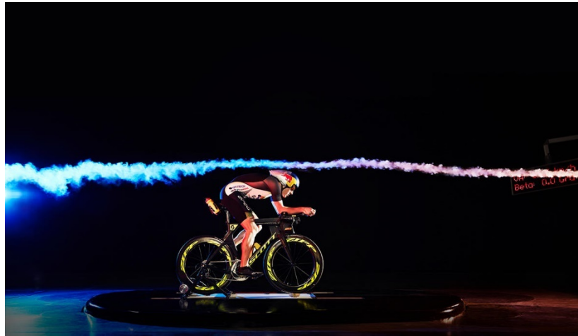
Figure 1: Optimisation of Cycling Position in a Wind Tunnel
