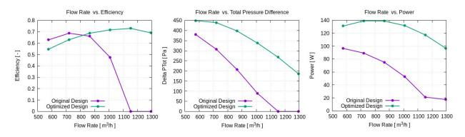
From the efficiency graph above, we can clearly see that the original design cannot operate in the new range of flow rates. This is the reason why there is a big difference in the objective function values. Additionally, the optimized design generates a higher pressure drop. In another words, the optimized design induces higher flow rate at the similar condition compared to the original design. The higher flow rate performance results in a higher power supply.
