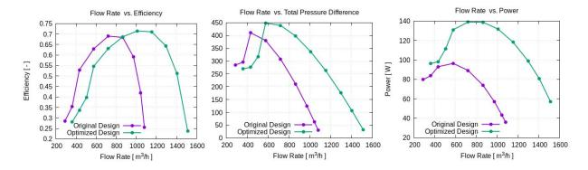
The complete maps tell us that the optimized design has a maximum air capacity over 1500m<sup>3</sup>/h, a peak efficiency is increased to 72%, a maximum pressure drop rises to 450 Pa and a working range is wider. The price of these significant improvements is 40W in a power supply.
