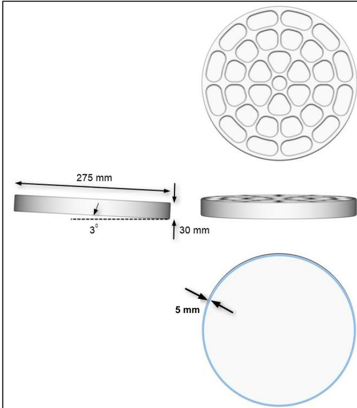
The mirror blank has a radius of 275 mm with a thickness of 30 mm.
