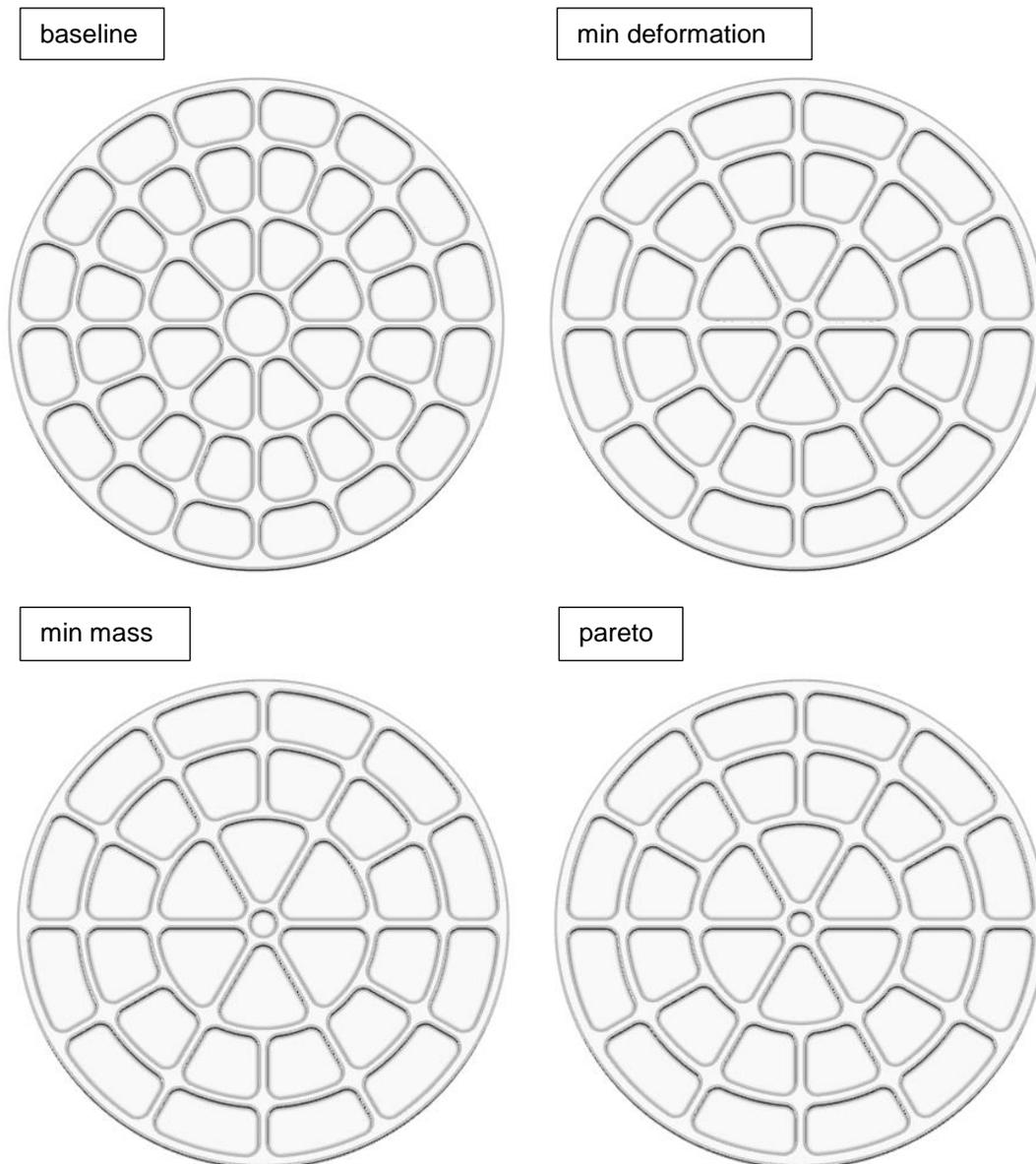
From the pictures above, it is surprisingly apparent that the three selected designs are quite similar in terms of geometry. All of them have a very small inner hole, and therefore hole corner radii, and all have 6 holes in the inner ring, while the baseline has large corner radii and 8 holes. Among these designs, the differences are mainly caused by different wall thicknesses between the holes and a different convexity, i.e., cross-sectional profile.
