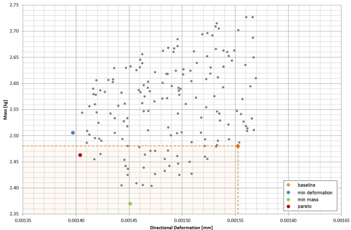
From this "Pareto frontier", three different designs were selected: the one with the lowest deformation, that has a slightly increased mass, the one with the lowest mass, that also has significantly lower deformation and finally, a compromise design that has a very low deformation, but also a slightly lower mass. This selection should simply illustrate that it is possible to select different designs from the generated database, depending on the emphasis in terms of the two considered objectives.
