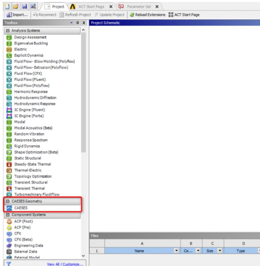
After the installation, the app will appear within the toolbox of ANSYS Workbench as a separate component system. It includes the CAESES Geometry, ANSYS Geometry and ANSYS Meshing components.
