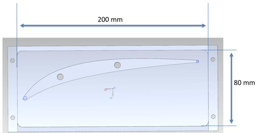
Fig. 3: Manufacturing constraints for the casing fixture
