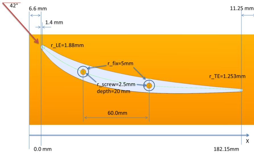
Fig. 2: Initial blade geometry (top) and axial positioning (bottom), including yellow domain for endwall profiling and manufacturing constraints (bottom)
