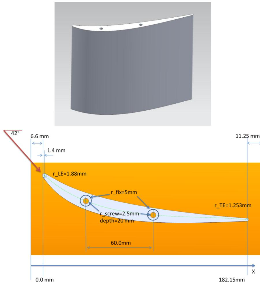
Fig. 2: Initial blade geometry (top) and axial positioning (bottom), including yellow domain for endwall profiling and manufacturing constraints (bottom)
